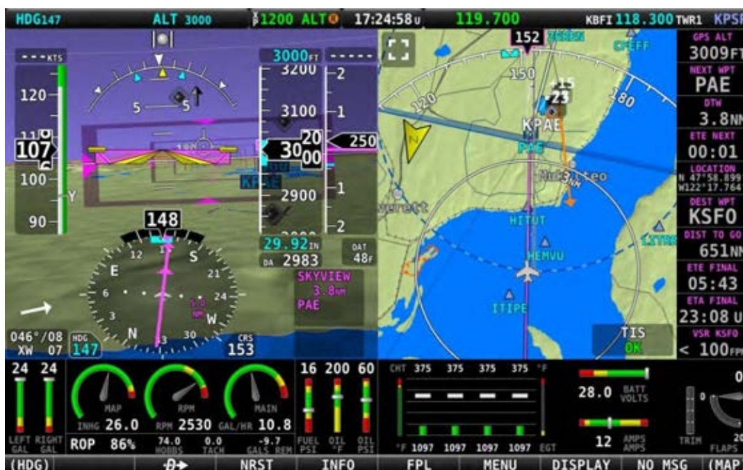
Figure 155 – Active Flight Plan: HSI and MAP Depictions
