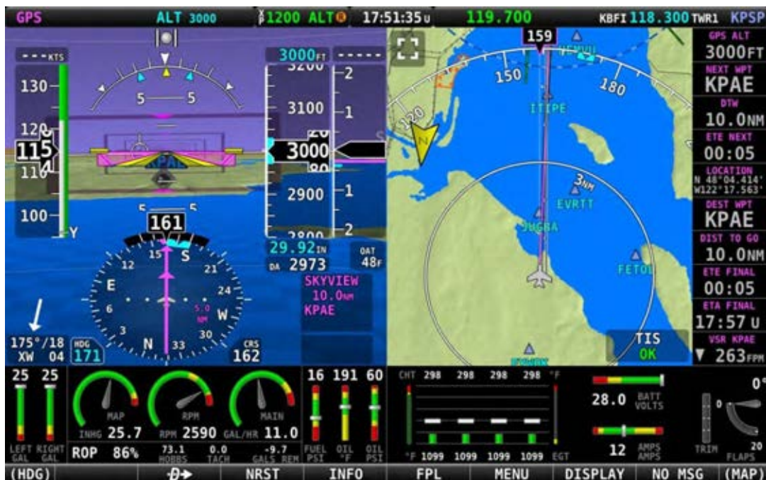
Figure 145 – Map/HSI with Navigation Active
