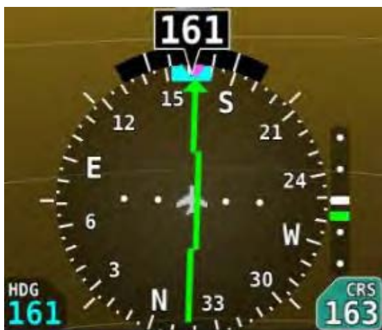
Figure 43 – HSI Example: Localizer
