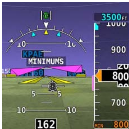
Figure 37 – MIN Bug and “MINIMUMS” Alert
