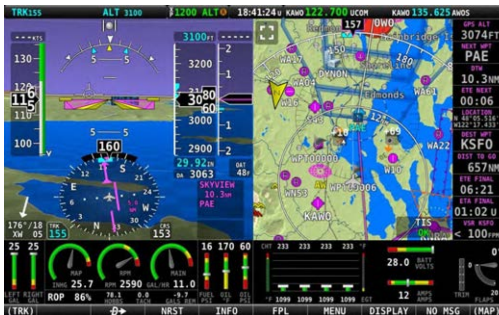
Figure 132 – MAP INFO COLUMN displayed on right side of screen
