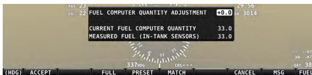
Figure 206 – Fuel Computer and Fuel Menu
