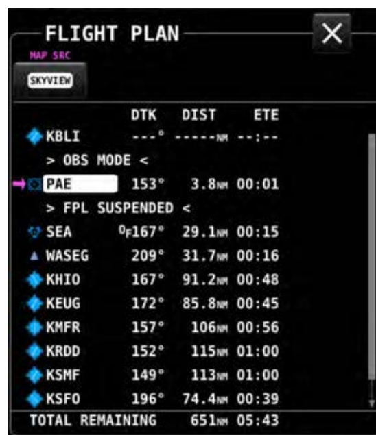
Figure 163 – OBS Mode Activated
