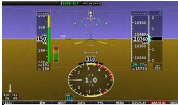
Figure 81 – G Meter in EFIS Presentation PFD
