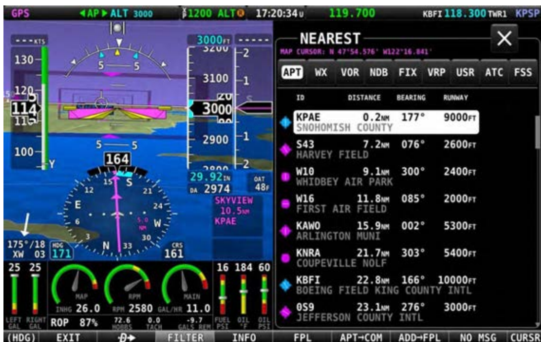
Figure 138 – Moving Map Nearest Window – Full Data
