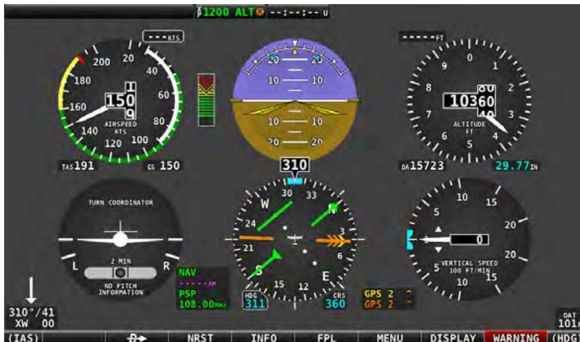
Figure 77 – Six Pack PFD Presentation, Synthetic Vision Disabled
