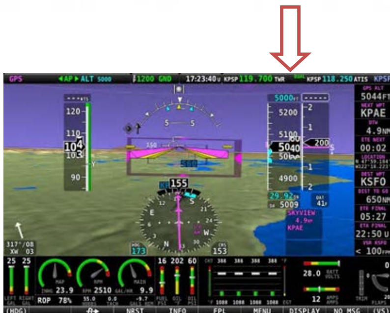
Figure 244 – SkyView Top Bar Com Radio Status Overview
