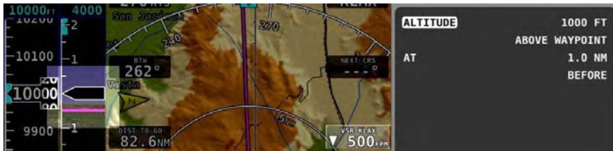
Figure 39 – Vertical Speed Required to Destination
