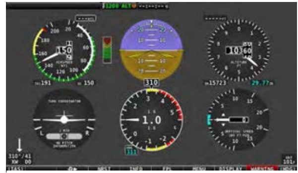
Figure 82 – G Meter in Six-Pack Presentation PFD
