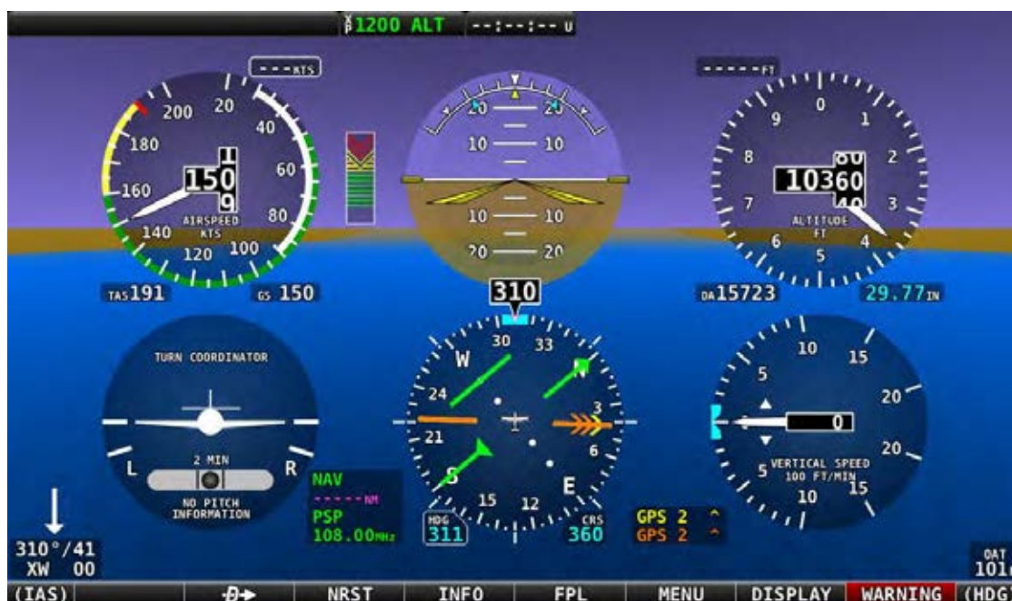
Figure 76 – Six Pack PFD Presentation, Synthetic Vision Enabled
