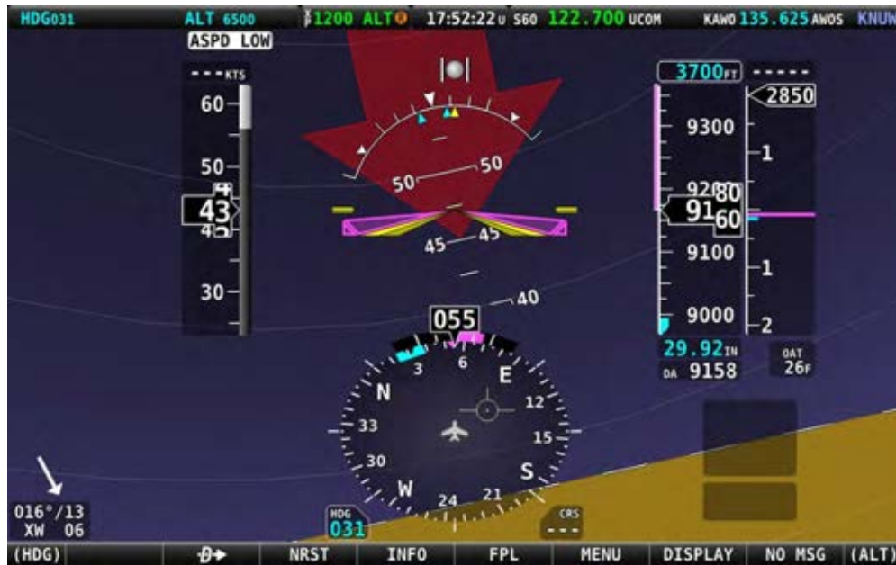
Figure 74 – Extreme Pitch Warning Indicator Arrows
