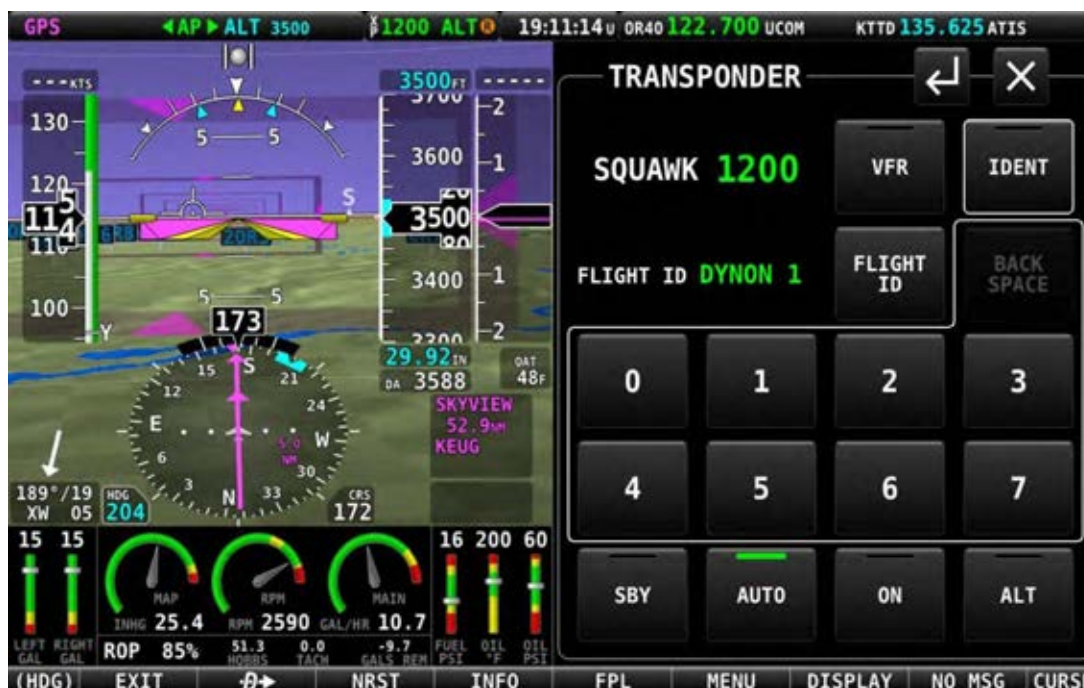
Figure 209 – TRANSPONDER control page
