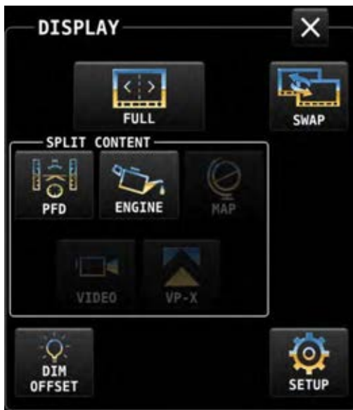
Figure 16 – DISPLAY menu showing the SWAP button
