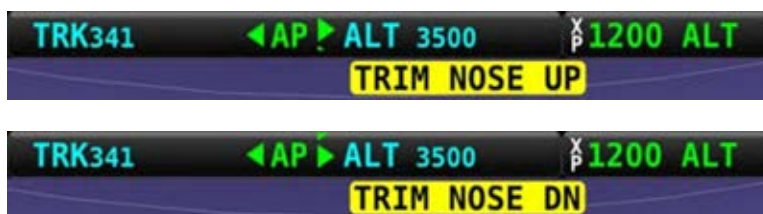
Figure 211 – Trim Nose Up and Down Alerts
