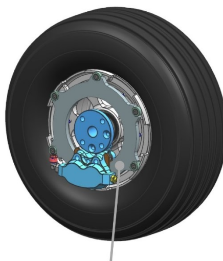
Brake disc type A8 (thickness 8 mm)
