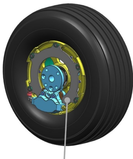
Brake disc type A3 (thickness 3 mm)
